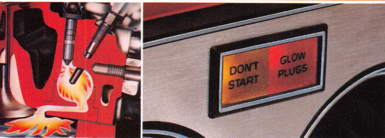
Electric glow plugs help provide efficient cold weather starting.
